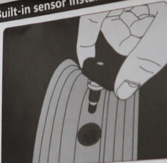
2 Mount the sensor into the valve.
