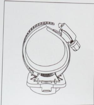
2. Screw the rod and loosen the bracket.
