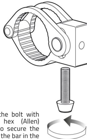
Tighten the bolt with an M5 hex (Allen) wrench to secure the clamp on the bar in the desired position.
