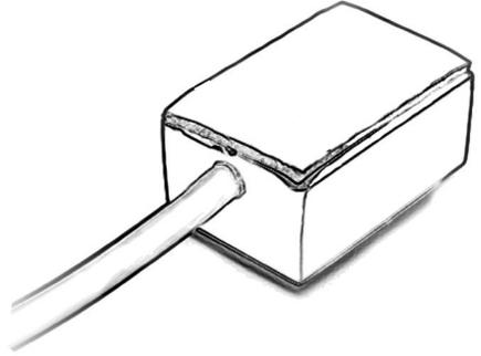
Make sure to leave the green plastic foil intact at the back of the display. If you remove the foil and expose the adhesive backing, you will not be able to remove the display from the mount later.
