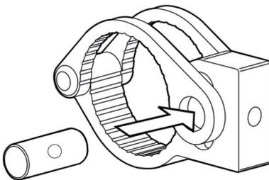
Slide the pin into place, making sure the threaded hole is aligned with the bolt hole.
