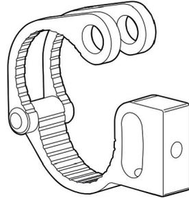
Wind the arm around the handlebar then close. If a plastic shim is used, rotate it to the correct position.
