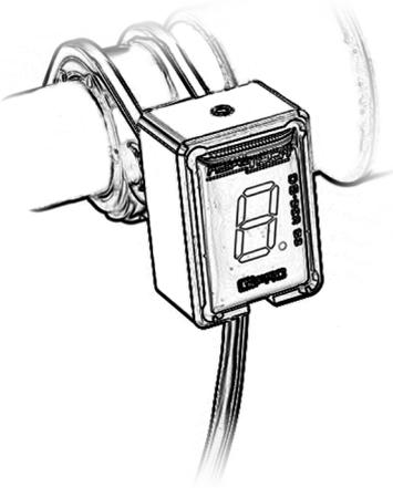
Place the Gipro into the housing then secure the unit in its place with the small Allen bolt at the top of the mount. Use the size 2 Allen key (supplied) to tighten the bolt gently. Do NOT overtighten as it may damage the Gipro.
