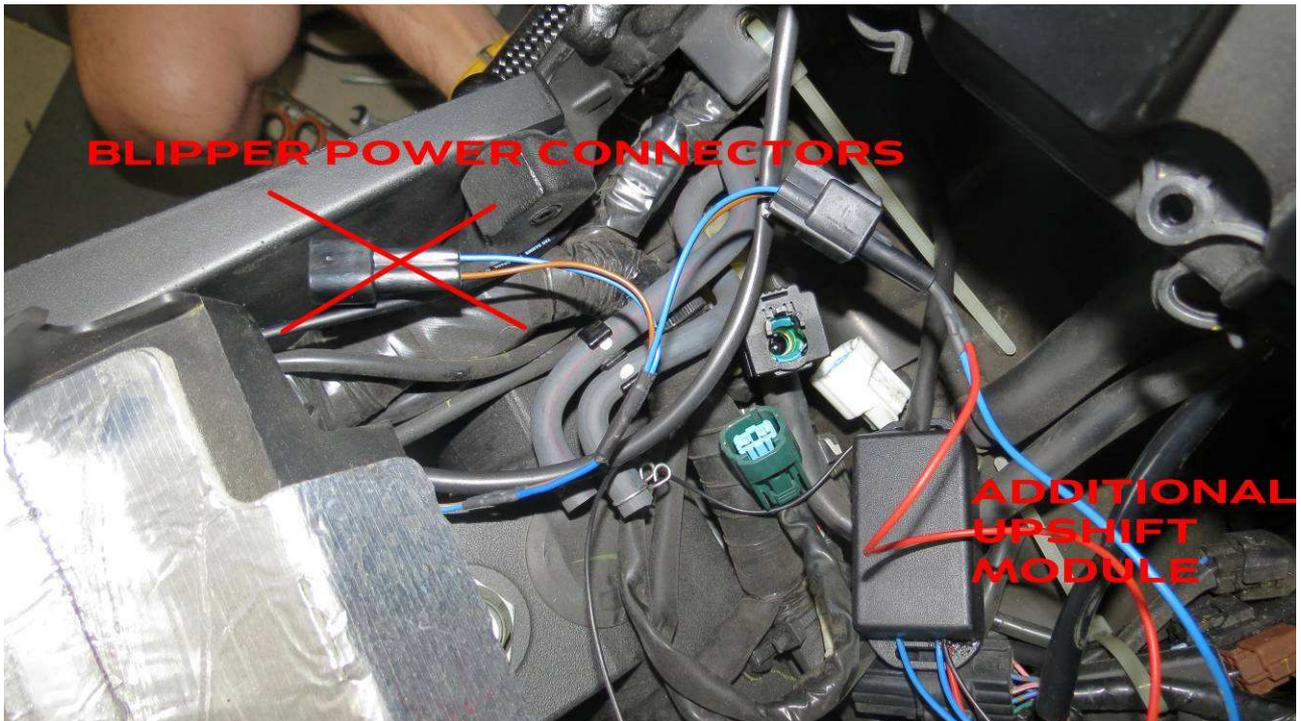
CONNECT THE BLIPPER UPSHIFT CONNECTOR TO THE ADDITIONAL MODULE FOR THE UPSHIFT. CONNECTORS AREN'T PROVIDED. YOU MUST CONNECT AS YOU LIKE THE 2 SAME COLOR WIRES.
