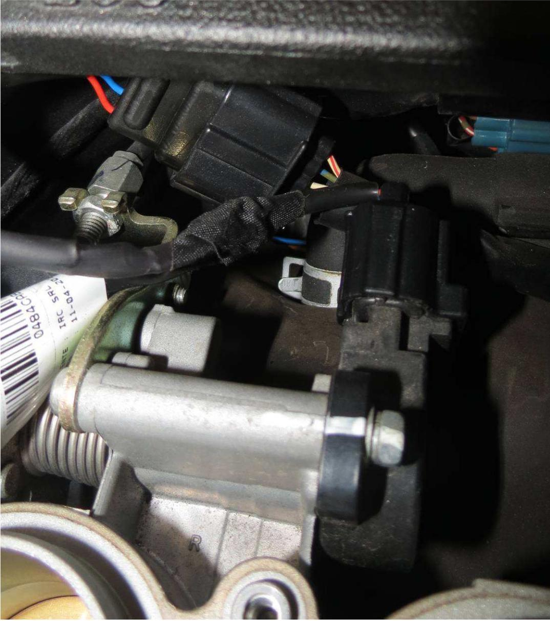
CONNECT THE POWER CONNECTOR OF THE BLIPPER TO THE ADDITIONAL MODULE FOR THE UPSHIFT
