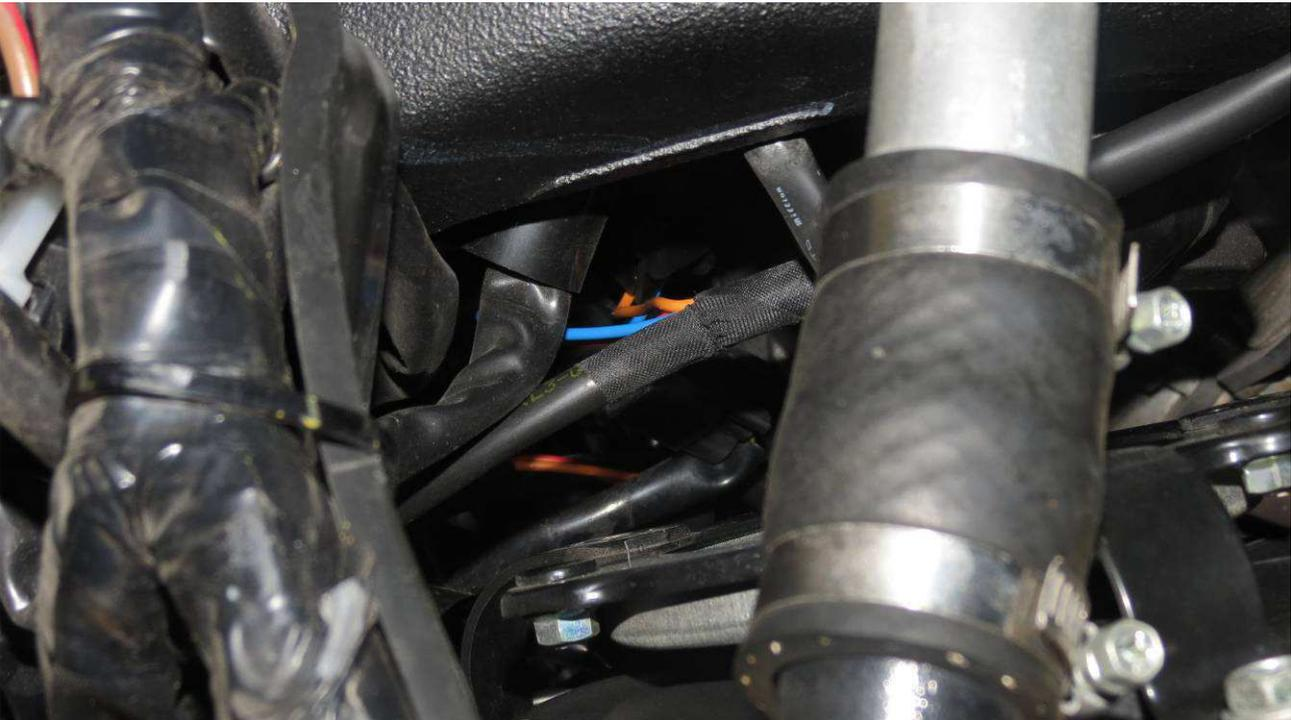
LOCATE THE APS CONNECTOR AND CONNECT IRC HARNESS (IT IS WHERE WIRES FROM THROTTLEGRIP ARRIVES. ON R6 ON THE LEFT, ON R1 ON THE RIGHT)
