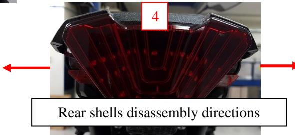
Rear shells disassembly directions
