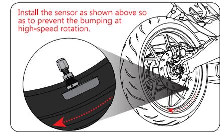
**Caution:** The installation direction of the sensor shown by the arrow shall be consistent with the self-rotation direction of the tire.
