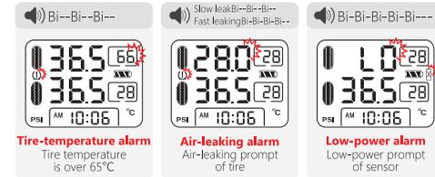
After the display alarms, press anywhere on the display to remove the prompt sound, and the flickering prompt will continue till the fault is removed
