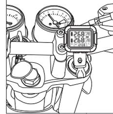
**Caution:** Turn on the power of the display and then install the sensor. Follow this step, and the data can be displayed at real time.
