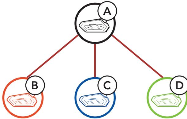
1. Press and hold the **Center Buttons** of two headsets for **5 seconds** until you hear a voice prompt, **"Intercom pairing"**.
