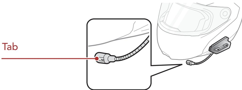
5. Align the arrows on the main unit and microphone cables and insert the microphone cable into the microphone connector.
