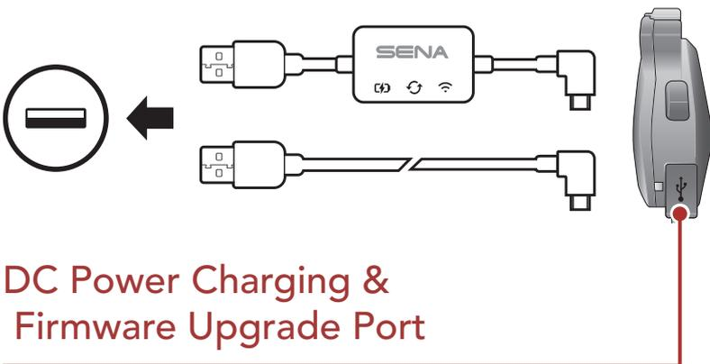
You can charge the headset by connecting the **WiFi Adapter** or a **USB Power & Data Cable (USB-C)**.
