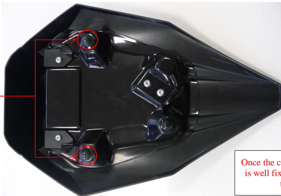
Once the cover fitted, check it is well fixed by trying to lift the front.
